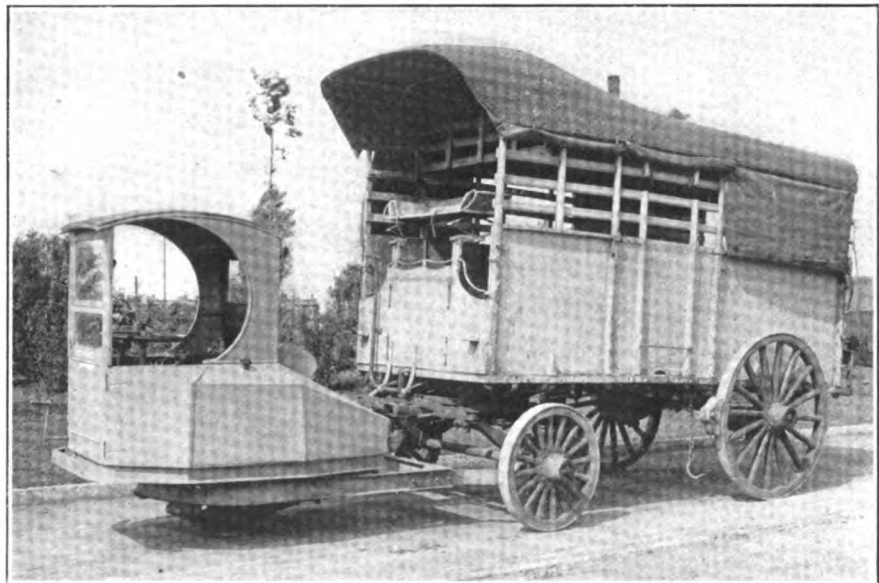
The iron horse, a one-wheel tractor adapted for hauling any ordinary animal vehicle with load of from one to five tons
